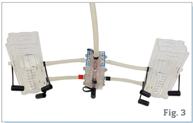
3. Fill the storage tanks with deionized or distilled water ( $\sigma < 2 \mu\text{S}/\text{cm}$ ) until water is coming out of the top connectors of the electrolyzer and travels into the tubing leading to the storage tanks.
